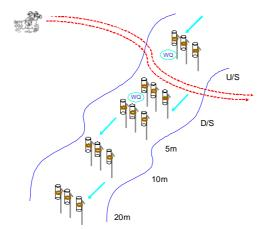
**Figure 3 Site Set Up.** Red lines indicate crossing. WQ = water quality conjection points, downstream (d/s) and upstream (u/s). Suspended sediment traps were placed three abreast of the thalwag (deepest point of the stream), at 1m upstream, then 1m, 5m, 10m and 20m downstream.
